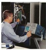
TekMate simplifies off-site service with virtually automatic setup and easy access to libraries of known-good waveforms stored on its 3.5-inch diskettes.
