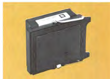
Graflok 2 Back, 4 x 5. Accepts Polaroid Land 4 x 5 film holder, standard cut-film holders, film-pack adapters, roll-film (120) holders, order 122-0931-00
